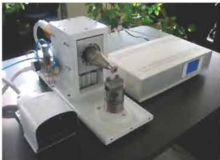
Ultrasonic welding equipment of textile materials 20kHz, 3000W
