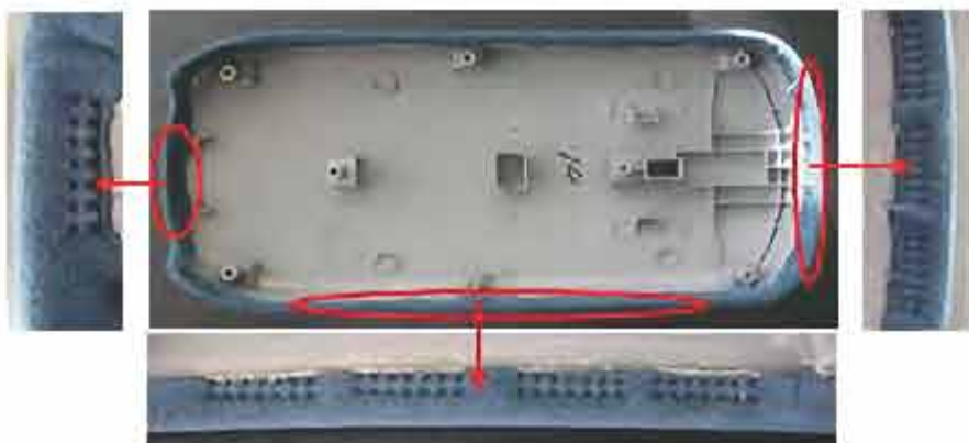
Elbow rests with fabric coating welded contour using ultrasounds
