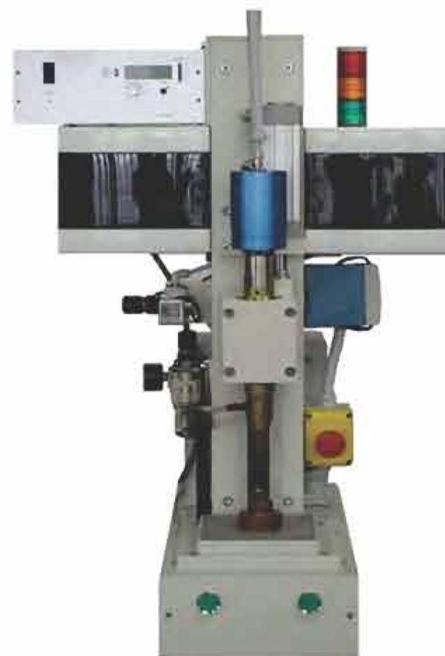
Hybrid welding equipment resistance welding and ultrasonic welding, 20kHz, 2500W
